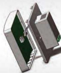
Carefully unplug the ribbon connector which is plugged in to the front half of the thermostat
